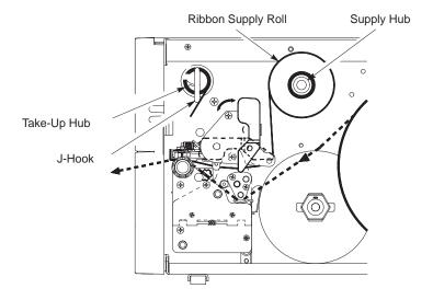
Make sure the ribbon roll is pushed up against the hub flange.
